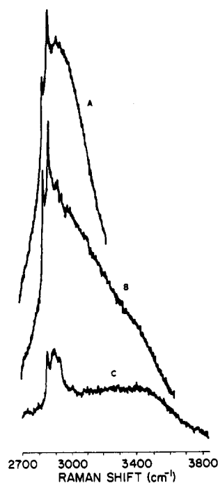
FIGURE 2: Changes in the raw Raman spectra for C18:0h-CBS in 2 M \text{Li}^+ with temperature: (A) 20.6 °C, (B) 41.7 °C, (C) 64 °C.
